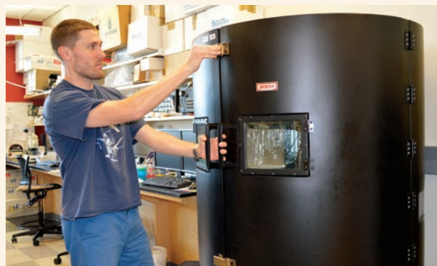
A graduate student operates the atomic force microscope in the Granzier Lab. During experiments, an enclosure protects the sensitive instrument from vibrations that would skew the measurements.
